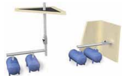
Horizontal mounting. Can be installed in the horizontal manifold for easy installation and access.
